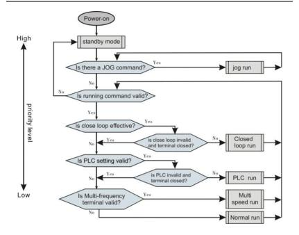
Fig. 4-2 Logical relationship diagram of inverter running status
