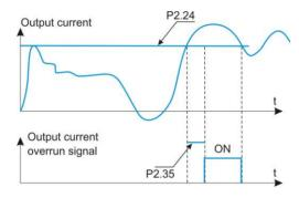
Fig. 6-14 Output current overrun detection
