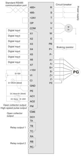
Fig. 3-6 Basic Wiring Diagram (NE90-4T0300G, NE90-4T0370G)
