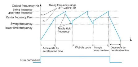
Figure 6-36 Schematic diagram of swing frequency
