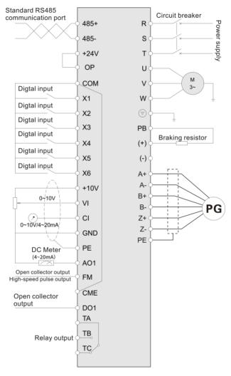
Fig. 3-5 Basic Wiring Diagram
