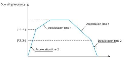
Fig. 6-12 Acceleration/deceleration switching
