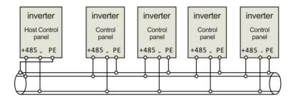
Fig. 3-15 Multi inverters communication
