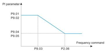
Fig. 6-32 PI parameters relationship diagram
