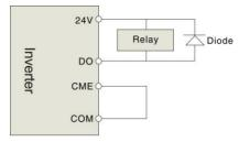
Figure 3-12 Schematic diagram of the digital output terminal wiring
