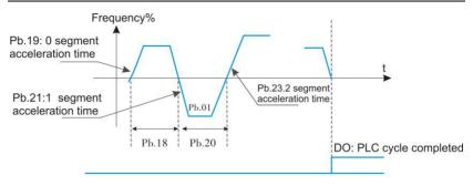
Figure 6-35 Simple PLC schematic
