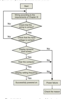
Fig. 4-1 Initial power-on operation of the inverter
