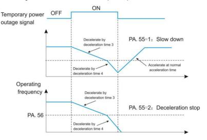
Figure 6-34 Level diagram of the FDT function
