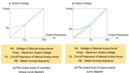
Fig.6-24 Manual torque boost
