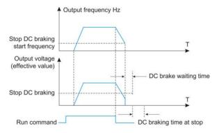
Fig. 6-02 Stop DC braking process
