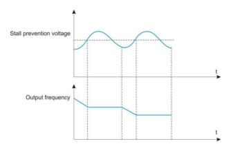
Figure 6-33 Over voltage stall function
