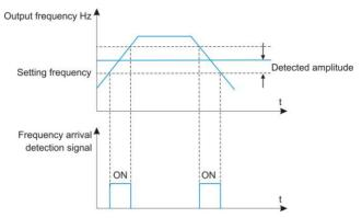
Fig. 6-09 Frequency arrival detection amplitude
