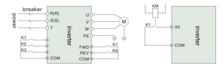
Figure 6-16 Multi-speed operation wiring diagram
