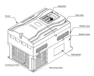
Fig 2-3 parts of Inverter
