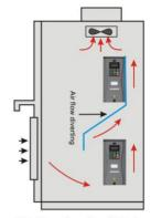
Figure 3-2 Mounting of multiple inverters
