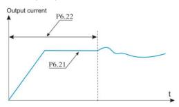
Fig.6-28 PID initial value function
