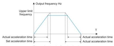
Fig. 6-1 Acceleration/Deceleration time
