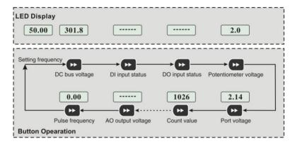
Fig.4-7 Example for running status data display operation
