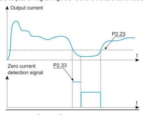
Fig. 6-13 Zero current detection
