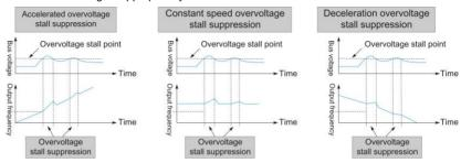
Figure 6-39 Schematic diagram of overvoltage stall action
