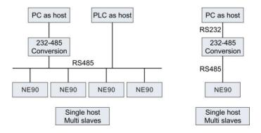
Figure 9-1 Schematic diagram of the unit network
